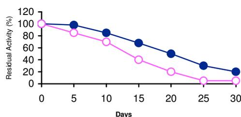
Fig. 4. Effect of storage on stability of free (○-○) and immobilized (●-●) lactate dehydrogenase at pH 7.5
